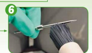
Please make sure that all brushes being used have no protruding metal wires as these may damage the spray gun. Please exclusively use recommended tools for cleaning only.
