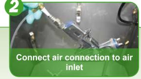
Please ensure that the spray gun is always placed in the correct position inside the washing chamber of self-contained washing machines. Make sure that no cleaning agent penetrates the air passages of the spray gun.
