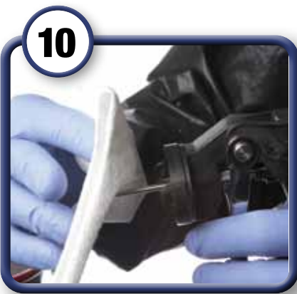
10 Wipe off any additional residue from the fluid needle.
