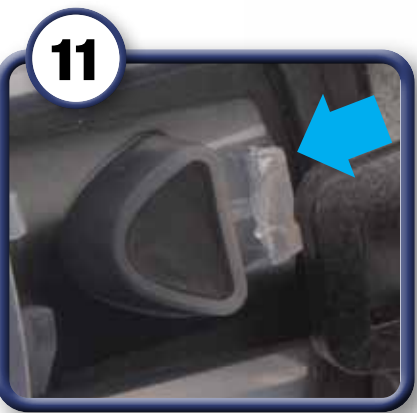
11 Inspect atomizing head for damage or wear which could result in fluid leaks or poor performance.
