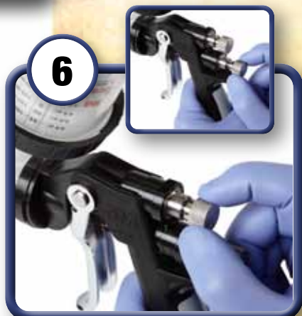
6 Adjust fan and fluid flow to achieve the desired size and wetness of the pattern. NOTE: when closing the fan adjustment completely it may be necessary to re-adjust the air flow control valve.
