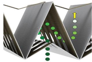
The forward momentum of the rapidly moving droplets separates them from the air stream which makes four quick and violent directional changes and so, deposits the droplets into the deep interior V pockets formed by each pleat.
