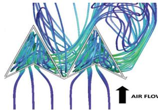
Consequently the static pressure increases only slowly with the accumulation of paint, enabling a uniform airflow around the parts that are being coated, and more importantly clean air environment for the sprayers.
