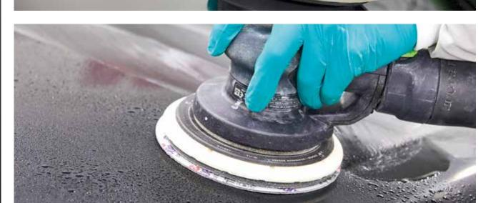
► Refine scratches with 3M<sup>™</sup> Trizact<sup>™</sup> Fine Finishing Disc 443SA, grade 3000, 150 mm on orbital sander.
