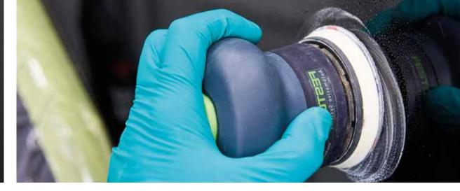
► Refine scratches with 3M<sup>™</sup> Trizact<sup>™</sup> Fine Finishing Disc 443SA, grade 8000, 75mm on orbital sander.
