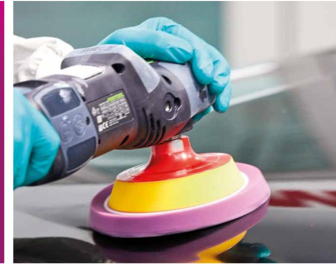
► Add a small amount of 3M<sup>™</sup> Perfect-It<sup>™</sup> 1-Step Finish Material to a purple foam pad on the rotary polisher.
