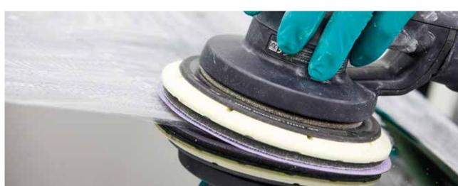
► Sand the area with 3M<sup>™</sup> Hookit<sup>™</sup> Purple Finishing Film Abrasive Disc 260L, grade P1500 - P2000.
