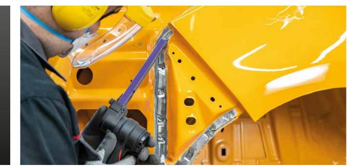
► Grind spot weld to remove weld from top panel. Note top panel thickness
