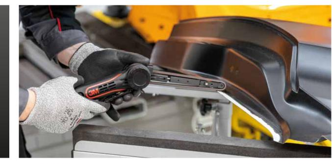
► Clean and prep remaining mating flanges on replacement panel with a Scotch-Brite™ Belt or Disc where necessary
