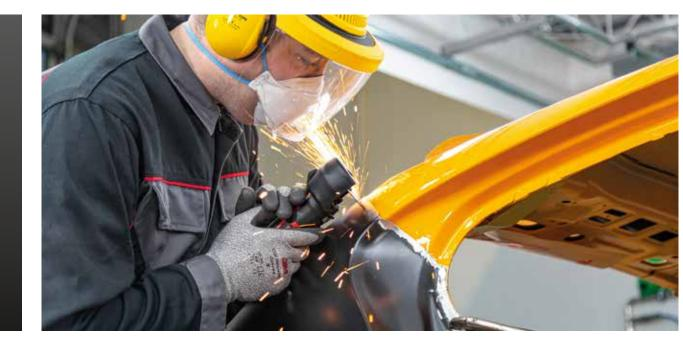
► Identify final cut line at the overlapping area of the pre cutted host and replacement panel
