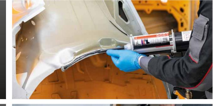
► Apply adhesive to mating flange areas on host panel and replacement panel as recommended from car manufacturer by covering all bare metal areas
