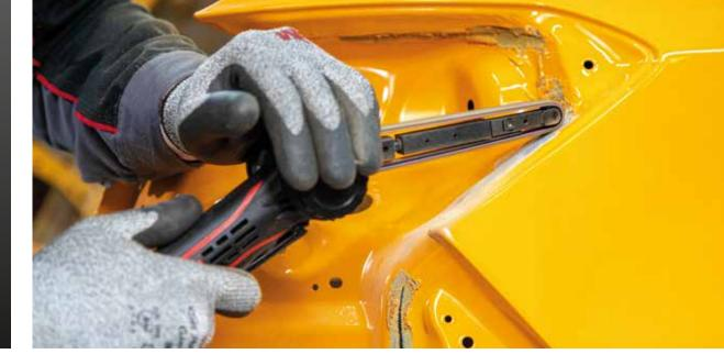
► Use Scotch-Brite<sup>™</sup> Belt to remove coatings and seam sealers in hard to reach areas and along pinch weld flanges to expose spot weld locations
