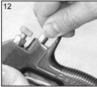
12. Fit Valve Seat to Gunbody.
