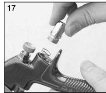
17. Replace Valve Spring by inserting small end of spring into gun, and screw in Housing (10).
