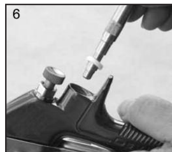
6. Retirer le support de la soupape.
