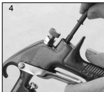
4. Retirer la soupape (11).
