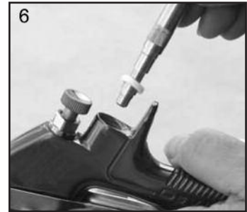
6. Remove Valve Seat.
