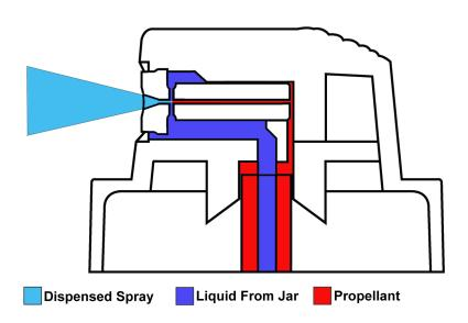
Preval has a proprietary technology that makes a highly controlled atomized spray from any liquid. When the button is pressed, propellant and liquid are mixed and dispensed as a spray at the nozzle by action of the venturi effect. Liquid from the jar is pulled up the tube as propellant travels across the holes in the red insert (inside the button). The propellant and liquid do not mix prior to being dispensed out of the nozzle.
