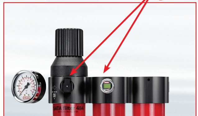
Upgrading an analog pressure gauge with a SATA adam 2 display with the help of a SATA dock (requires adapter from G 1/4 male thread to G 1/8 female thread, Part No. 677023)
