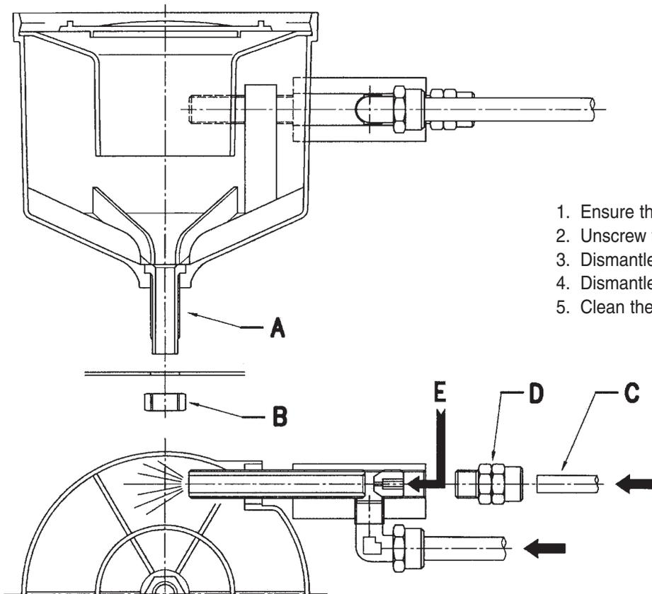
1. Ensure that the discharge hose **A** is not obstructed.
