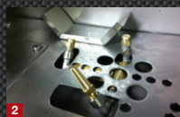
2 Place the nozzle provided in the fitting
