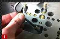
1 Remove the spray blank
