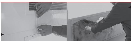
Each transparent anti-static polypropylene layer is treated with paint adhesion to trap overspray.
