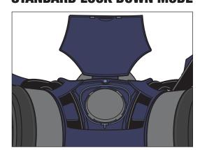
To lock the straps in position, open the valve cover by pulling up on the latch. Position straps underneath the tabs of the strap channel. Close and snap shut the valve cover.
