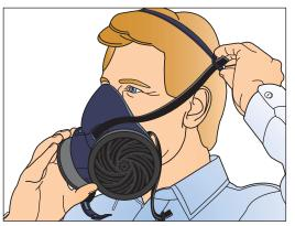
First adjust head cradle then place respirator under the chin and pull the cradle to the top of the head so it rests on the crown.
