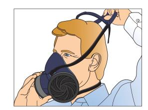
Adjust head cradle then pull the cradle to the top of the head so it rests on the crown.
