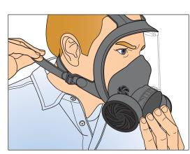
Push facepiece onto face and chin with one hand and position for most comfortable and secure seal while pulling and tightening neck tab of harness with other hand. Repeat for other neck tab. For easiest, most secure and best fit, always adjust neck harness tabs first before tightening top harness tabs.
