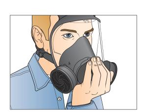
Positive Pressure Seal Check: Cover the exhalation valve vent without pressing too hard against face, then exhale gently to create a slight positive pressure. If air leakage is detected, re-adjust the position of the facepiece and the tension of head harness and repeat the seal check until leakage is eliminated.
