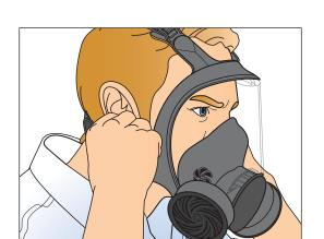
Grab lower lengths of head harness with each hand, just above each adjustment buckle, and while positioning chin in flange, pull harness over the head.
