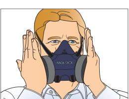
**Negative Pressure Seal Check: Cover** both cartridges without pressing too hard against face, and gently inhale and hold your breath. The facepiece should slightly collapse. If air leakage is detected, re-adjust the position of the facepiece and the tension of both headstraps and repeat the seal check until leakage is eliminated.
