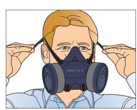
Tighten top straps first then the lower neck straps until you have a very snug and leak-free fit. Facepiece should not be loose or slide up or down the nose. Tighten by pulling on ends or loosen by pushing out on buckle tab. Do not overtighten. Further tighten top straps if necessary.
