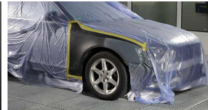
► Before applying the base and clear coats, further cut the masking film and attach it to previous contour and aperture masking.
