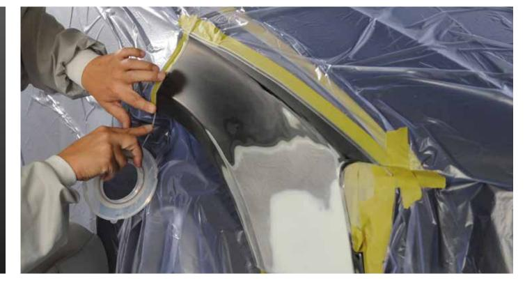
► For best results, apply 3M<sup>™</sup> Smooth Transition Tape on top of the 3M Masking tape to allow a smooth transition of primer edges.
