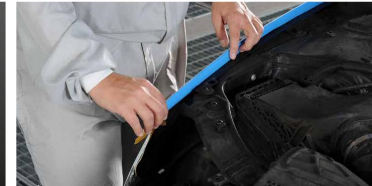
► Prepare the area for paint application, ensuring sufficient space to allow for smooth transitions and avoid hard edges.
