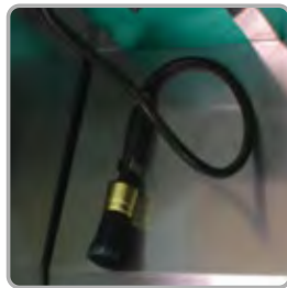
Brush for washing the gun exterior areas
