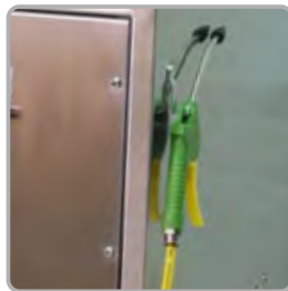
Gun with coupling to clean interior areas
