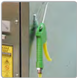
Blowgun for drying the gun interior areas.
