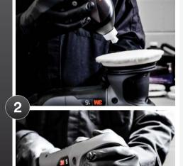
► Apply the compound to the pad in a circular motion by using the cap from the bottle to help spread a small amount of compound throughout the pad. When applying compound to a new pad, its recommended starting at speed setting 1 for a few seconds, to ensure the pad is loaded evenly with compoun before starting the task.
