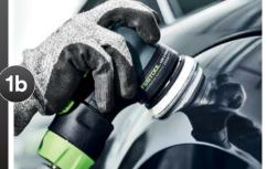
► Sand the area with a 3M<sup>TM</sup> Hookit<sup>TM</sup> Purple Finishing Film Abrasive Disc 260L, grade P1500, 3" (75 mm). Use disc with a soft interface pad. Remove all panel defects and match texture to adjacent OEM panels. Wipe panel clean.
