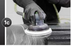
► Sand the area with a 3M<sup>™</sup> Hookit<sup>™</sup> Purple Finishing Film Abrasive Disc 260L, grade P1500 - P2000, 6" (150 mm). Use disc with a soft interface pad. Remove all panel defects and match texture to adjacent OEM panels. Wipe panel clean.
