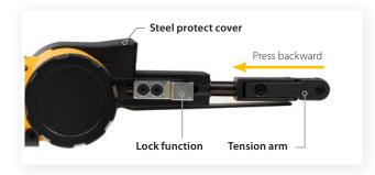
In order to release the belt, press the tension arm towards the steel protect cover to release lock function. Open the protect cover by loosening the cover knob.
