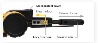
Replace with a new belt. Close the protect cover and tighten the cover knob. Fixate the new belt by pressing the lock towards the steel cover – which releases the tension arm forward.
